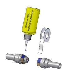
WE RECOMMEND TO SEAL THE FITTINGS WITH BRASS THREADS ONLY BY CEMENT, TEFLON TAPE OR TEFLON THREAD
