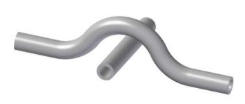
CROSSING OF PIPELINE IS TO BE MADE USING SPECIAL ELEMENTS DESIGNED FOR THIS PURPOSE
